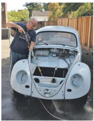
Hays Englehart, Beetle rehab project leader, powerwashes front bay, from which spare tire had been removed. All of the mechanical-repair work was done at his home in Moraga.
